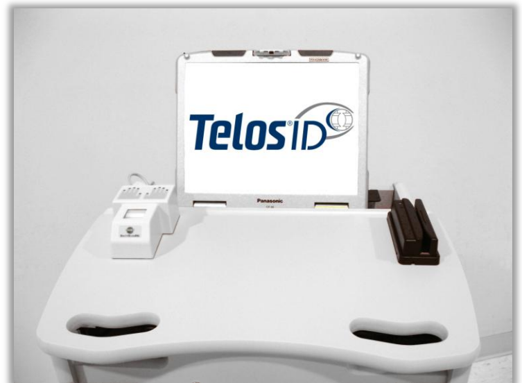
The check-in console at FedExField showing the fingerprint swipe on the left and the card swipe on the right. The efficiency of the MAAC system has increased the speed with which security officials can verify the credentials of employees as they enter the facility.
